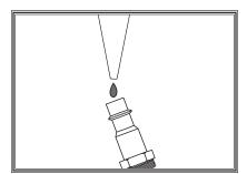
Figure 7. Lubricating nailer via air inlet.
